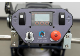
Centralized control unit with carbon monoxide monitor
