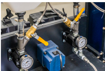
2 BALL VALVES TO FLUSH PUMP LINES
