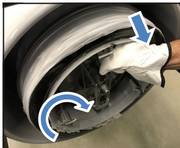
9- Pull and rotate the retaining pins and insert them into their seats.
