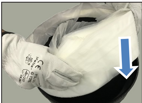
4- Insert the new Infinity Bag with the inner part facing upwards.
