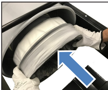
8- Insert the container with the Infinity Bag.
