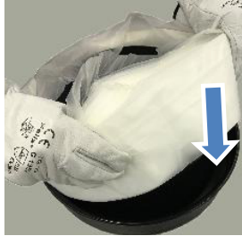
3- Insert the new Infinity Bag with the inner part facing upwards.
