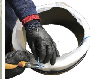
4- Cut and remove the Infinity Bag closing bands.
