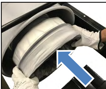
8- Insert the container with the Infinity Bag.
