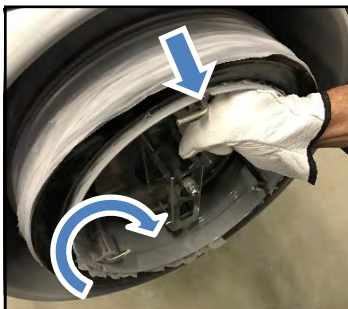
2- Pull and rotate the retaining pins of the Infinity bag container in order to unfasten them.
