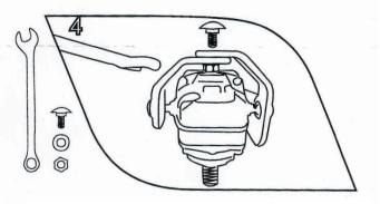
Use the short screw to assemble the two parts of the SpeediEdge.
