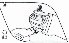
Feel the two plastic rings on both spherical bearings.
