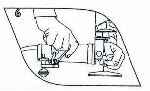
The last step is to calibrate the SpeediEdge assembly - Place on flat surface
