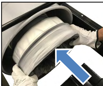
8- Insert the container with the Infinity Max Bag.
