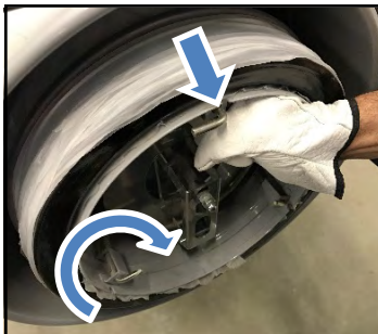
2- Pull and rotate the retaining pins of the Infinity Max bag container in order to unfasten them.
