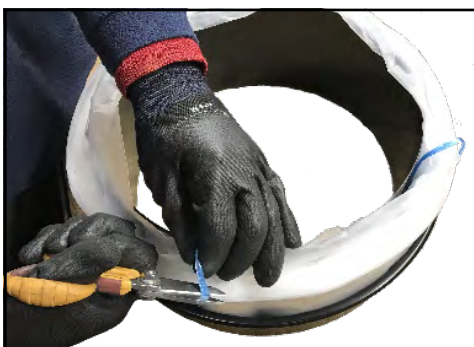
5- Cut and remove the Infinity Max Bag closing bands.
