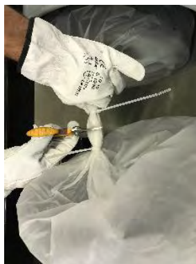
2 - Cut the strip between the two bands.
