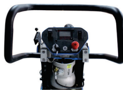
Centralized control unit with carbon monoxide monitor
