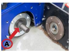
8. Using the guide pins (A), reattach the bearing plate to the machine using the bolts previously removed. Be sure the bearing is seated onto the shaft. It may be helpful to lower the machine so that the drum is touching the ground taking the load off the shaft allowing easier alignment of the holes.
