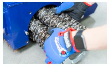
7. Slide the new drum back onto the shaft. Be sure that the drum is fully seated onto the driving plate, and the spacer (A) is fully seated against the drum.
