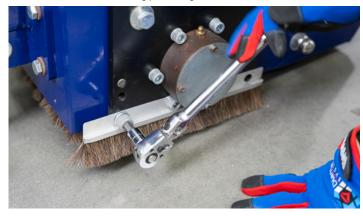
3. Remove the top 2 bolts using an M18 Wrench.
