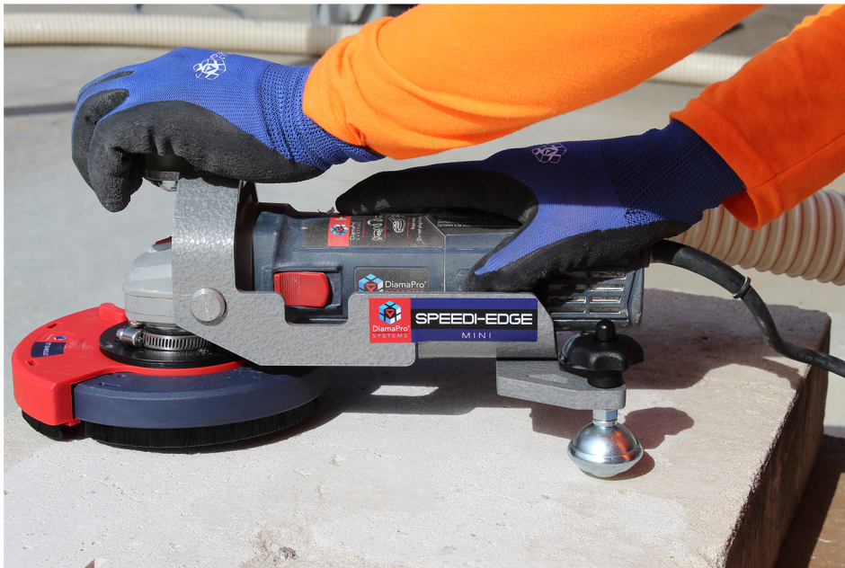
Speedi Edge in use with a 5" HGX-5 hand grinder.
